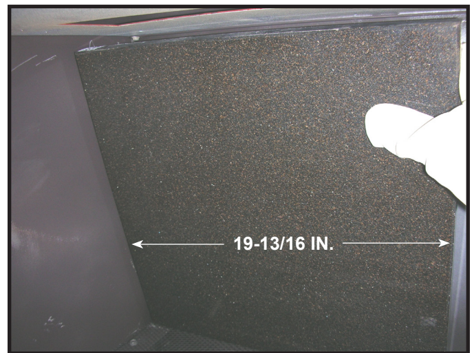
Figure 6. Placing Back Panel Piece.
